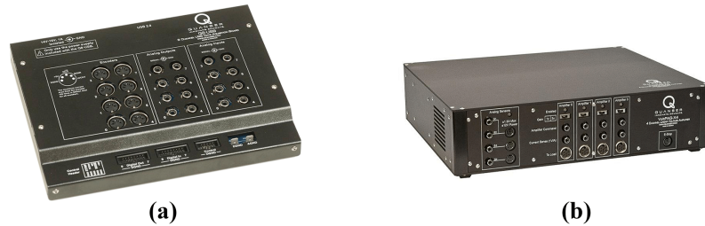
Figure 2.13 : (a) Quanser Q8-USB data acquisition device. (b) Quanser VoltPAQ-X4 linear voltage amplifier.
