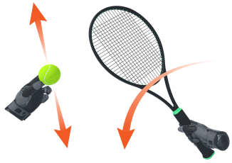
Figure 5: The weight and inertia of rigid-body objects can be rendered through fluctuations in squeeze.
